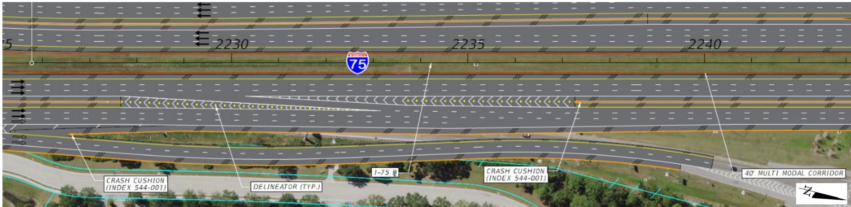
Figure 4.5: Slip Ramp at University Parkway - Egress
