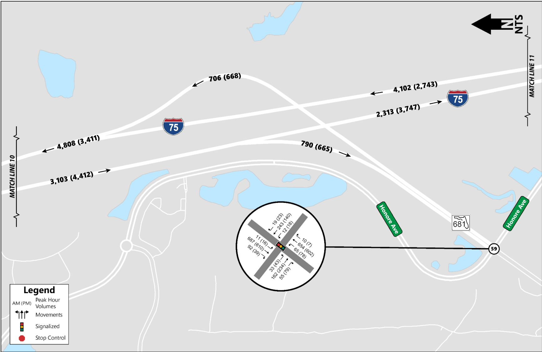
Figure 6-25 Existing Year (2019) DDHVs and Peak-Hour Turning Movement Volumes - I-75/SR 681 Interchange
